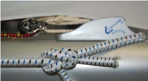
**25** Tie off the bungee around the boom forward of the cleat with a bowline.
